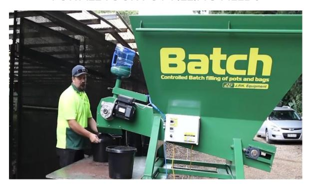
BATCH, Flat & Pot Filler by JPH is designed to take the backbreaking labour out of pot filling in the horticultural industry. It's a fast, reliable and repeatable way of filling almost any type of pot, container, hanging baskets and nursery flatswith the correct mix of soil and fertilizer. It designed to be fast, filling an average 8"/400mm pot in under 10seconds, allowing you to do hundreds of uniform pots in an hour.
